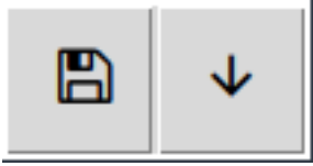
Figure 1.5: An example of the Familiarity principle. At first glance, which button looks more like it would be responsible for 'saving'?
